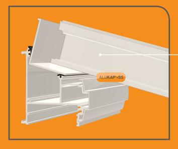
4. Cut the first ALUKAP®-SS High Span/Low Profile base bar to the correct length to allow it to rest between the top and bottom ALUKAP®-SS Bar Caps. Measure the bolt fixing position from the end of the ALUKAP®-SS base bar for drilling a hole through the ALUKAP®-SS Span base bar and down through the bold flange on the ALUKAP®-SS Eaves Beam and Wall Plate. This will vary between 40mm and 70mm depending on the pitch).
