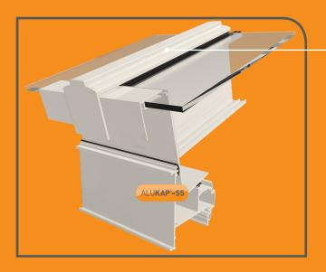
16. Now carefully cut the ALUKAP®-SS Top Bar Top Cap to the accurate length required for a perfect aesthetically pleasing finish. For gable end or wall abutments use the ALUKAP®-SS Gable Bar or Wall Bar Top Cap. Snap the ALUKAP®-SS Top Bar Top Caps on to the ALUKAP®-SS Top Bar Base Caps along the whole length of the bar. Use a suitable rubber / plastic headed hammer for this action and avoid heavy impact, to avoid damage to the ALUKAP®-SS bar and the glazing materials.
