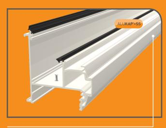
2. Cut the ALUKAP®-SS Eaves Beam to the overall external width of your roof structure. Screw/bolt securely to the top of your window frame or post bracket with suitable stainless steel fixings. Fit ALUKAP® bar gasket on to the base rail and upright rail.
