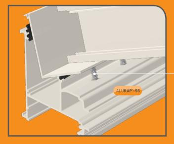
9. Slot the 6mm M6 bolts through both sides of each bar, top and bottom, and then lightly screw the M6 nuts on to the four M6 bolts for each ALUKAP®-SS Span Base Bar. When you are happy that the positions are all correct, tighten up the nuts.
