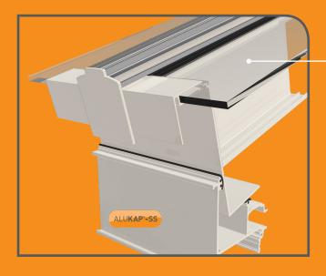
15. Then offer up the next glazing panel and repeat the procedure above to fix the next intermediate ALUKAP®-SS Top Bar Base Cap between the first and second glazing panel. Then continue along the rest of the roof until all glazing panels are secured.
